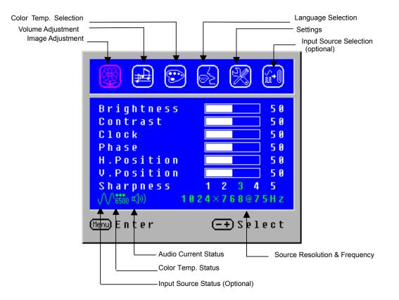
Repeat above steps for changing the setting of other functions. The following is a list of the OSD sub-menus for the LCD monitor.
